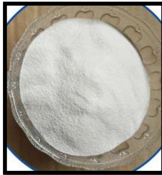
Figure 1: Insulating additive form – tiny ceramic inert gas filled microspheres [4]
